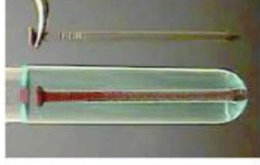
fig-11(a): Iron nail dipped in copper sulphate solution
